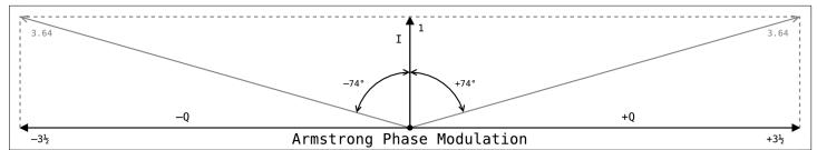
In the image above is the phase deviation graph during Luma & Chroma modulation. While the I channel remains static with a DC carrier level of 1 the Q channel when modulated by  $M_{\lambda}$ ,  $M_B$  &  $M_R$  will peak at Tan( $\pm 74^\circ$ )= $\pm 3\frac{1}{2}$  producing a peak envelope modulation of 3.64.
