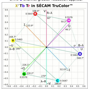
A method for converting  $\Sigma HS\lambda$  Color with a modified Luma ( $\lambda$ ) to analog Color TV  $\lambda UV$  to balance for better Chroma (UV) matrixing.
