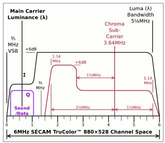
weighting of the luminance so an equilateral hexagon is created on the Cartesian grid, however U has been further reduced by  $\sim 3^{3}_{4}\%$  in relation to V so both U & V peak at ±1%, to eliminate ~3.9% peak difference. The PM sound sub-carriers are on the Q channel of the main carrier.
