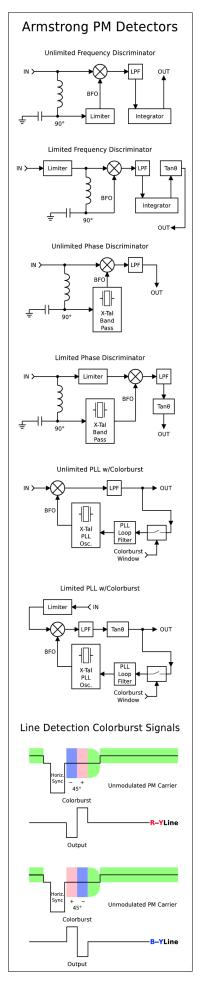
The 4<sup>th</sup> example is like the 3<sup>rd</sup> but operates on a fully limited signal for additional noise reduction but the Tan $\theta$  characteristic is lost. Wave shaping must be done to restore Tan $\theta$ . Examples 5 & 6 are like 3 & 4 respectfully except that the crystal ringing oscillator is replaced with a PLL version locked to a colorburst signal on the back porch of the horizontal sync.
