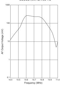
$\begin{array}{l} Input = 100 dB \mu \\ fdev. = \pm 50 kHz \\ fmod. = 1 kHz \\ Vcc = 5.0 V \end{array}$
