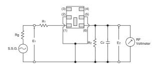
$\begin{array}{lll} Rg = 50\Omega & R1 = 280\Omega \pm 5\% & R2 = 330\Omega \pm 5\% \\ C2 = 10 \pm 2 \ pF & (Including stray capacitance and Input capacitance of RF voltmeter) \\ E1: S.S.G. Output Voltage \end{array}$
