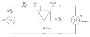
Rg+R1 =R2 : Input/Output Impedance
