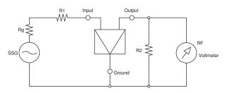
Rg+R1 =R2 : Input/Output Impedance
