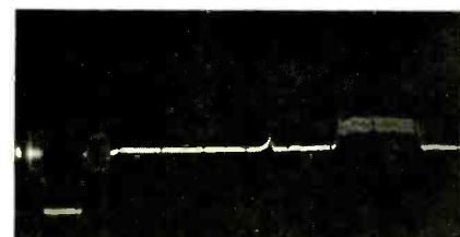
FIG. 4—THE SINGLE VIDEO LINE. (All waveform photos made with the Tektronix T935 oscilloscope.)
