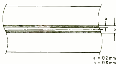
FIG. 7—CONTROL TRACKS may be used for automatic selection, synchronization or other purposes.
