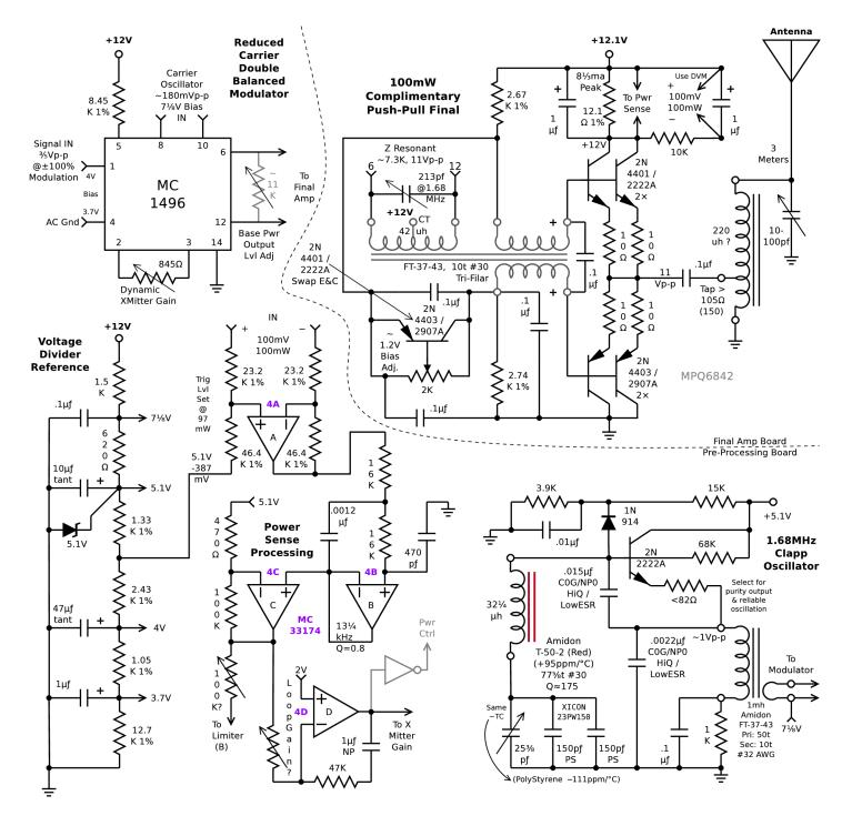
Since the finals low impedance output addresses antenna equalization and negative modulation not exceed -100% for receiver IF does bandwidth compensation the need for modulations greater than this provided by the MC1496 are unnecessary. This custom designed modulator is better suited for the setup on page Its better drive capability for the finals 13. better immunity from impedance provides changes caused by the antenna load.
