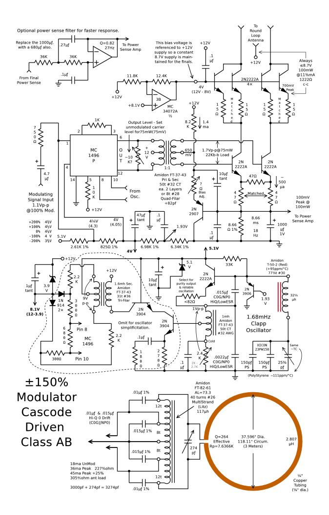
eliminate crossover distortion. It is necessary to use a center tapped 470 $\mu$ h choke with a 1K resistive load to properly observe any distortion on the scope. The high Q antenna will also filter out any RF harmonics but any distortion can make the -100% modulation transition point rough.
