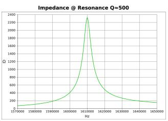
and adding in the other neutralizing factors the running Q could be >500 with a neutralized Z of 21/3K. This value of output Z has been created by Re + r'e of ~100 $\Omega$  combined with the initial output Z of ~800 $\Omega$  to create enough negative resistance needed to produce the necessary feedback for oscillation.
