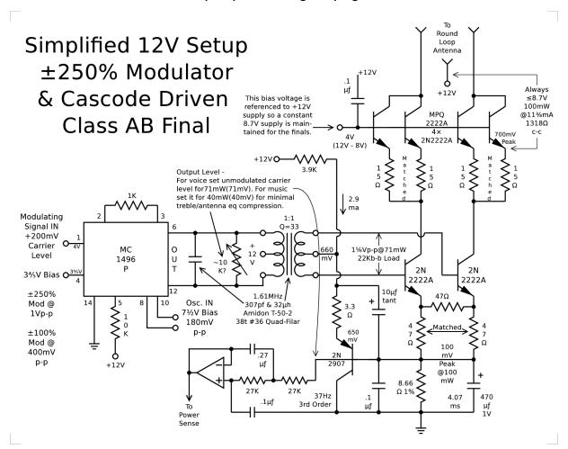
In lieu of using a Vactrol based dynamic pre-emphasis control in the case one can't be obtained here is a fully electronic version that offers tighter controlled attack/decay timing performance of ~9ms/~130ms respectively.
