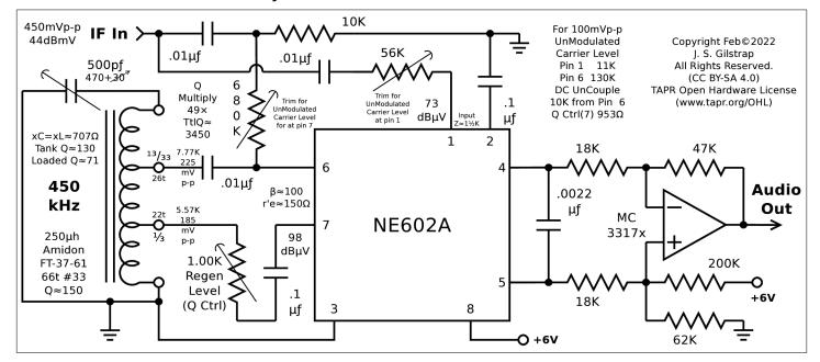
A potential variation could be to increase feedback till critical for synchronized oscillation once adequate signal level is reached. The blend would be completely transparent. It could be automatic in that the feedback level is directly coupled to detected signal level. This would basicly be full synchronous detection but with an appearant instant acquisition time.
