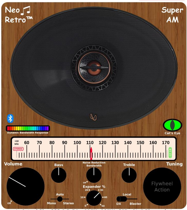
**↑ Actual Size 222.1 D.P.I. 11"H×10"W×8"D,** <sup>5</sup>/<sub>16</sub>" **Plywood ↑ 2 Ports:** ~45Hz, 3cm Dia, 16cm Long × 2 (1" PVC, I.D. 1.181", Sched. 20)
