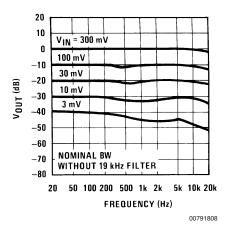
FIGURE 3. Output vs Frequency
